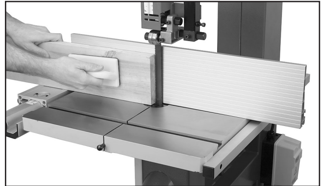
Figure 45. Example of resawing lumber.
